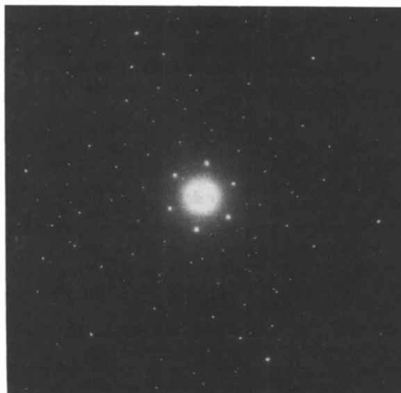
Fig. 1. Electron diffraction pattern from boric acid observed at T \leq 128 K.
